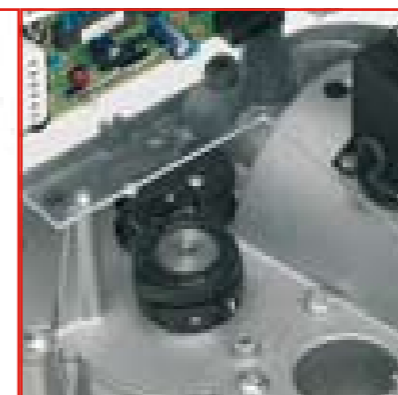
Limit switches adjustables inward
